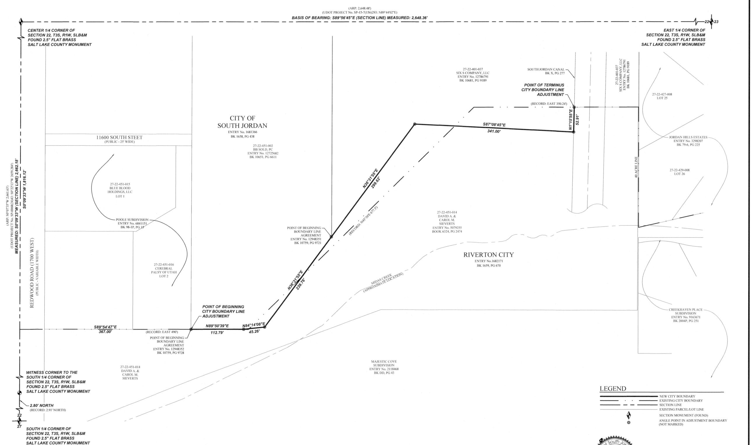
A CITY OF SOUTH JORDAN AND RIVERTON CITY BOUNDARY ADJUSTMENT IN THE SE1/4 OF SECTION 22, TOWNSHIP 3 SOUTH, RANGE 1 WEST, SALT LAKE BASE AND MERIDIAN (THE BASIS OF BEARING BEING S89°56'45"E MEASURED FROM THE CENTER OUARTER CORNER TO THE EAST QUARTER CORNER OF SAID SECTION 22.), BEING MORE PARTICULARLY DESCRIBED AS FOLLOWS:
